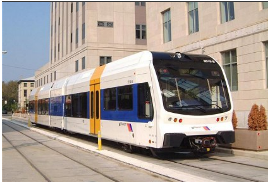
Figure 1 NJT River Line Diesel Light Rail Vehicle
